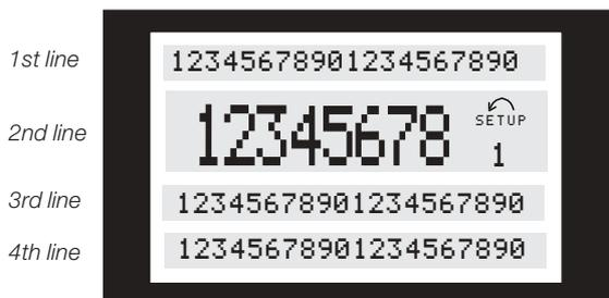
**1st line** shows up to 3 measurements continuously in normal operating status or a text which explains the 2nd line.
