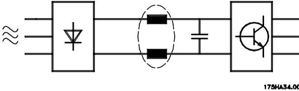
To ensure low, harmonic currents, FCM 300 has intermediate circuit coils as standard..
