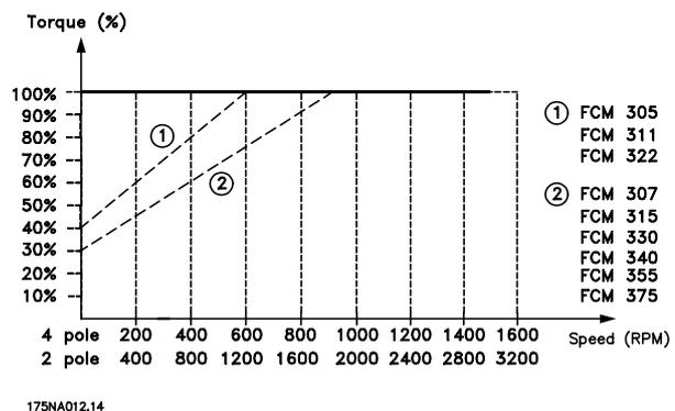
Nominal torque (100%) can be yielded up to 15 min and at a duty cycle up to 25% at low speed.
