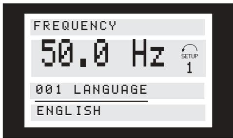
The 3rd line of the display shows the parameter number and name, while the status/value of the selected parameter is shown in line 4.
