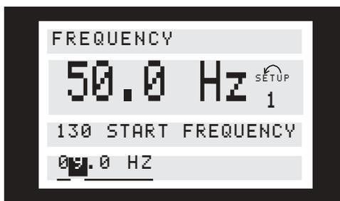
Then the chosen digit is changed infinitely variably by means of the [+/-] keys:
